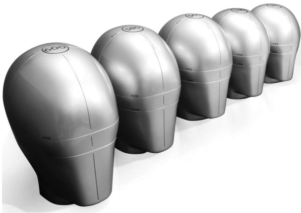
Figure 9. Chinese Headforms. The first set of 10 headforms for use in designing Asian-fit products.
